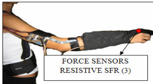
Figure 3. Arm sensor application- Force sensors resistive SFR (3)
