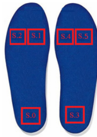
Fig.4. The positioning of the sensor on the insole
