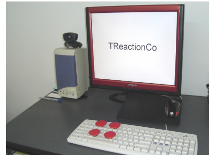
Fig. 1 – Software and adapted keyboard, in order to measure the reaction time
