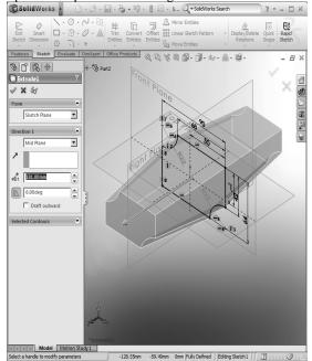
Fig. 16 "Draft" option of "Extrude" command
