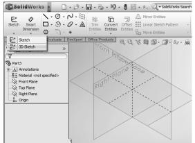
Fig. 12 Positioning of "3D Sketch"
