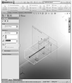
Fig. 15 Dynamic visualization of "Extrude" command
