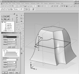
Fig. 9 Parameters of "Crown" option
