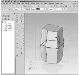
Fig. 8 "Draft" option of "Protrusion" command
