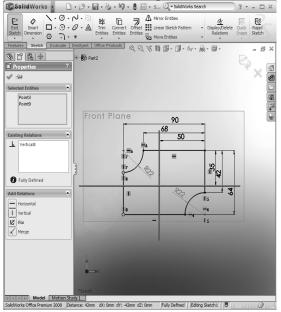
Fig. 13 Inserting constraints for points
