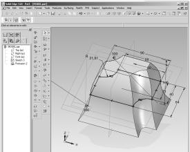
Fig. 10 Dynamic editing of "Protrusion"
