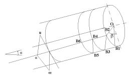
Fig.6. Diagram for studying the material particle trajectory along the screen
