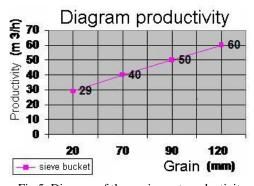
Fig.5. Diagram of the equipment productivity expressed in  $m^3/h$
