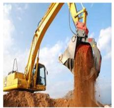
Fig.1. Equipment - rotary screening bucket attachable to the excavator arm
