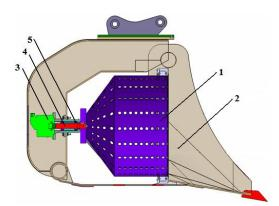
Figure 3. Equipment with rotary screening bucket – side view 1-screen, 2- bucket, 3-rotary hydro-static engine, 4-turning shaft, 5-bearing
