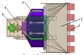
Figure 4. Equipment with rotary screening bucket – top view 1-tooth, 2-bucket, 3-screen, 4-engine, 5-bolt
