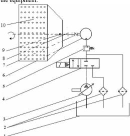
Fig.2. Hydraulic Kinematic Diagram 1-tank; 2-filters; 3- variable-delivery pump; 4-distribuitor; 5-safety valve; 6- rotary hydraulic engine; 7-safety clutch; 8-shaft; 9-bearings; 10-bucket
