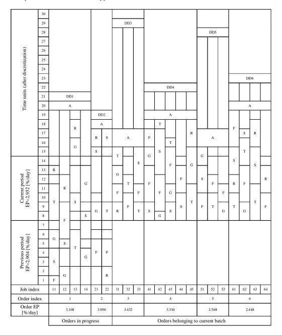
Fig. 2 Scheduling diagram - before simulation case F - milling, R - grinding, S - turning, T - thermal treatment, G - drilling, A - assembling
