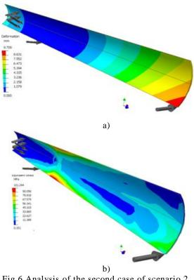
Fig.6 Analysis of the second case of scenario 2 a) deformation; b) equivalent stress Table 2 Results of FEM analysis
