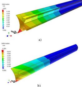
Fig. 4. Deformations of the two blades a) type A; b) type B.
