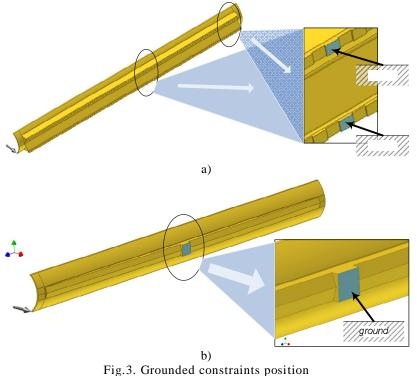
a) on type A blade; b) on type B blade.
