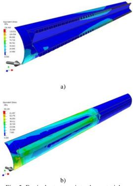
Fig. 5. Equivalent stress into the material of the two blades a) type A; b) type B (first case study).
