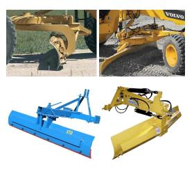
Fig. 2. Constructive solutions for the grader's blade (Caterpillar, Volvo, John Deere models)
