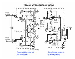
Fig. 1 Typical oil metering and export diagram
