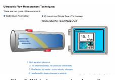
Fig. 3 Wide beam technology flow measurement
