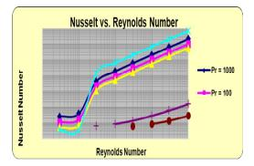
Fig. 11 Internal Flow Correlation for Heavy oil viscosity at 20<sup>o</sup>C
