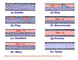
Fig. 7 Multiphase flow patterns in horizontal pipe.
