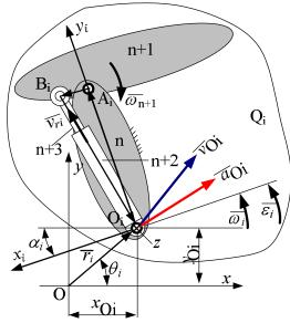
Fig. 3. Due to increased current stroke of the hydraulic cylinder, the item "n" rotates clockwise.
