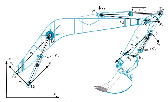
Fig. 5. Reporting systems in case of an excavator with reverse bucket.
