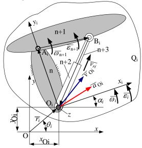
Fig. 2. Due to increased current stroke of hydraulic cylinder, the item "n" rotates counterclockwise.
