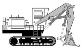
Fig. 1. Hydraulic Excavator with loading equipment
