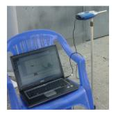
Fig. 3. Sonometer Solo 0.1 dB with laptop during measurements
