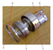
Figure. 2. Photo experimental gasodynamic radial sonic generator: Photo of the overall radial type generator gazodinamic: 1 - resonator;
