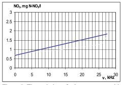
Figure 9. The variation of nitrate content with the ultrasound frequency
