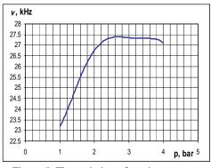
Figure 5. The variation of sonic generator acoustic frequency with the input pressure
