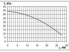
Figure 6. The variation of turbidity with the ultrasound frequency
