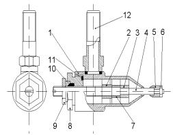
Figure 1. The sonic generator scheme: 1-air nozzle; 2,3-cross support; 4-rod; 5-resonator; 6screw-nut M2,5; 7-sleeve; 8-cover; 9-locking nut; 10-gasket; 11- ring; 12-fitting.
