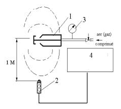
Figure 4. The acoustic testing diagram: 1- sonic generator, 2-microphone, 3-manometer, 4testing system "Brüel & Kjær"
