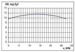
Figure 8. The variation of dissolved oxygen with the ultrasound frequency
