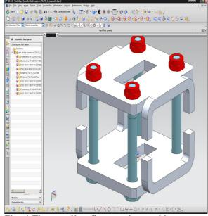
Fig. 4 The coupling flange subassembly.
