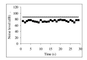
Fig. 11 Sound level in the command cabin while the ship is idling with generator engine generator; (---)-87dB, limit value [8]
