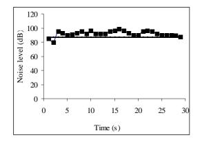
Fig. 8 The sound level on the main deck while the ship is running (---)-87dB, limit value [8]
