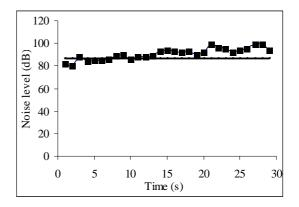
Fig. 13 Sound level inside the rest area while the ship performs the mooring manoeuvre; (---)-87dB, limit value [8]
