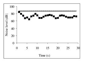
the ship performs the mooring manoeuvre (—)-87dB, limit value [8]
