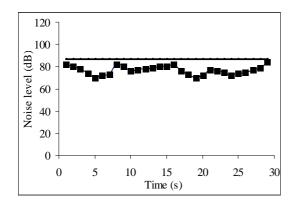
Fig. 12 Sound level inside the rest area while the ship is running;(--)-87dB, limit value [8]
