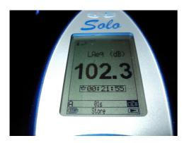
Fig. 4 Sonometer Blue Solo
