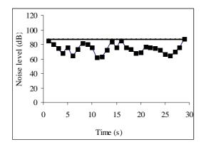
Fig. 6 The sound level on the navigation bridge while Fig. 7 The sound level on the navigation bridge while the ship starts from the shore (—)-87dB, limit value [8]
