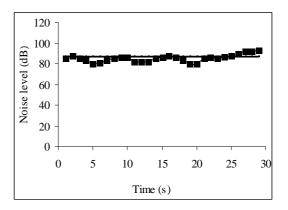
Fig. 9 The sound level on the main deck while the ship performs the mooring manoeuvre (---)-87dB, limit value [8]
