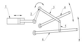
Figure 3.1. Schematic representation of the suspension mechanism[11]
