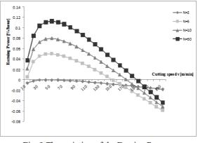
Fig. 2 The variation of the Earning Power depending on cutting speed
