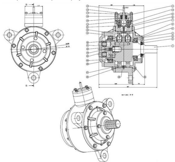
Fig. 5 Assembly drawing of the hydrostatic engine with variable engine capacity:
