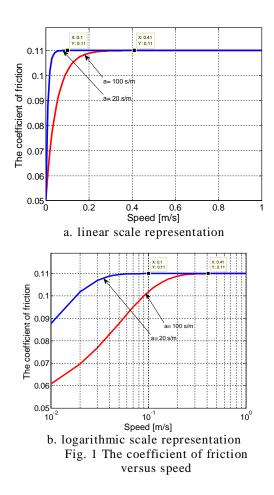
Experimental measurements have shown that for a higher speed of 150 mm/s, the maximum value of the coefficient of friction for any type of coating based on PTFE is reached.
