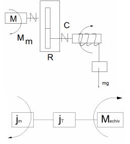
Fig. 3 - Scheme to reduce inertial elements
