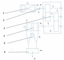
Fig. 1- The physical model of tower crane hoisting mechanism (Scheme kinematics) 1 -Motor drive, 2 - Coupling, 3 - Reductor, 4 -Reel, 5 -Tackle, 6 - Lifting weight
