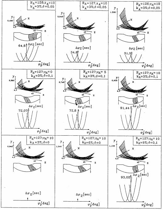
Fig. 1 [7] Numerical results related to the location of contact (contact pattern for a distance between the flanks  $\Delta = 15 \mu m$ ) for a cylindrical worm gearing with the following parameters: A=160mm; m=5mm; u=51/2; ZK1- gearing type; d<sub>1</sub>=12.5·5=62.5mm; d<sub>a1</sub>=73.5mm; d<sub>2</sub>=255mm; d<sub>a2</sub>=268.5mm; d<sub>a4</sub>=275mm; b<sub>2</sub>=45mm.
