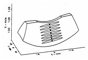
Fig. 4 [3] Contact pattern on the surface of the worm wheel
