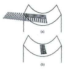
Fig. 2 [2] Contact pattern for the worm gearing ZE: a) Unchanged worm gearing;
