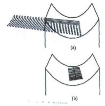
Fig. 3 [2] Contact pattern for the worm gearing ZK:
