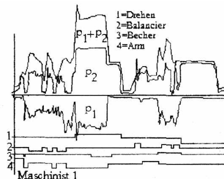
Figure 1. The instant power in the working cycle for 1.2 mc excavator
