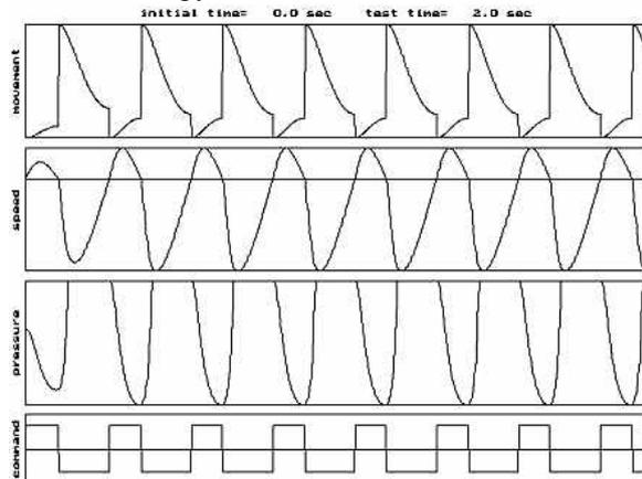
Figure 2. Hydraulic device parameters temporal evolution for 2 sec. beginning at  $t_0 = 0$
