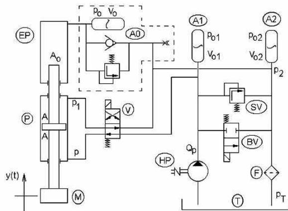
Figure 1. Schematic diagram of hydraulic vibratory device
