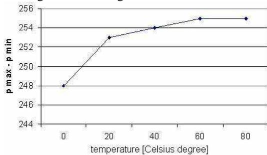
Figure 4. Pressure limits evolution as a function of the fluid temperature
