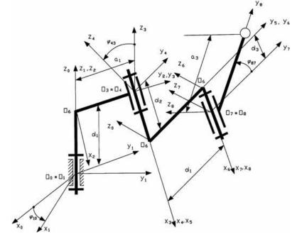
Figure 2. Kinematics positioning chain  $R \perp R ||R|$
