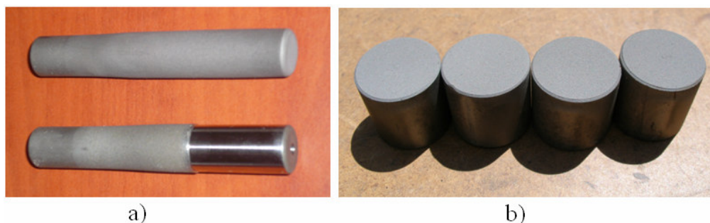
Figure 4. Pictures of the samples coated with a) 316L stainless steel as coated and machined, b) WC-Co coatings
